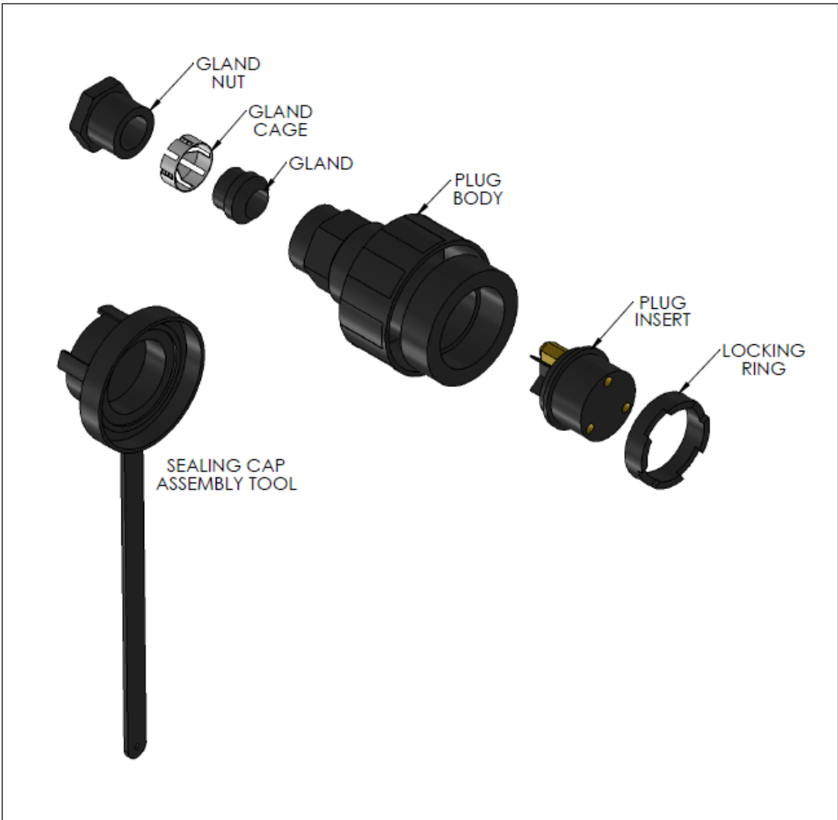
Figure 13. Disassembled Plug Connector
