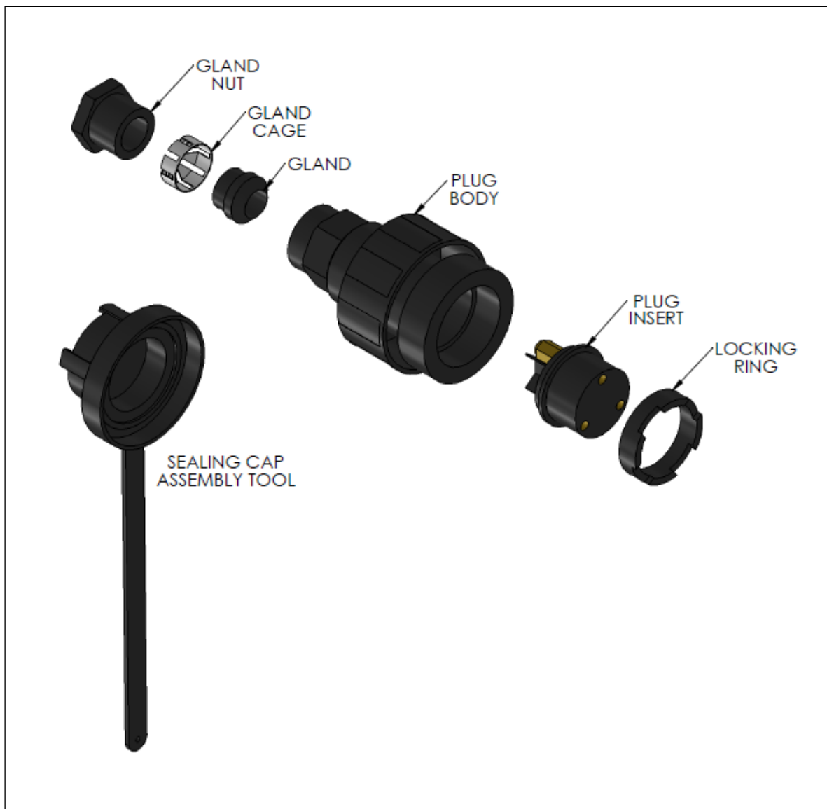
Figure 15. Disassembled Plug Connector
