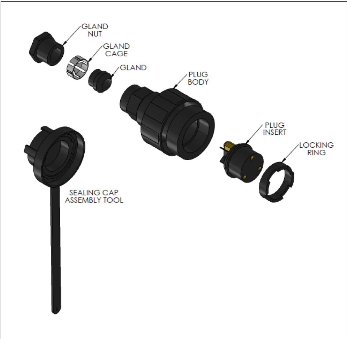
Figure 13. Disassembled Plug Connector
