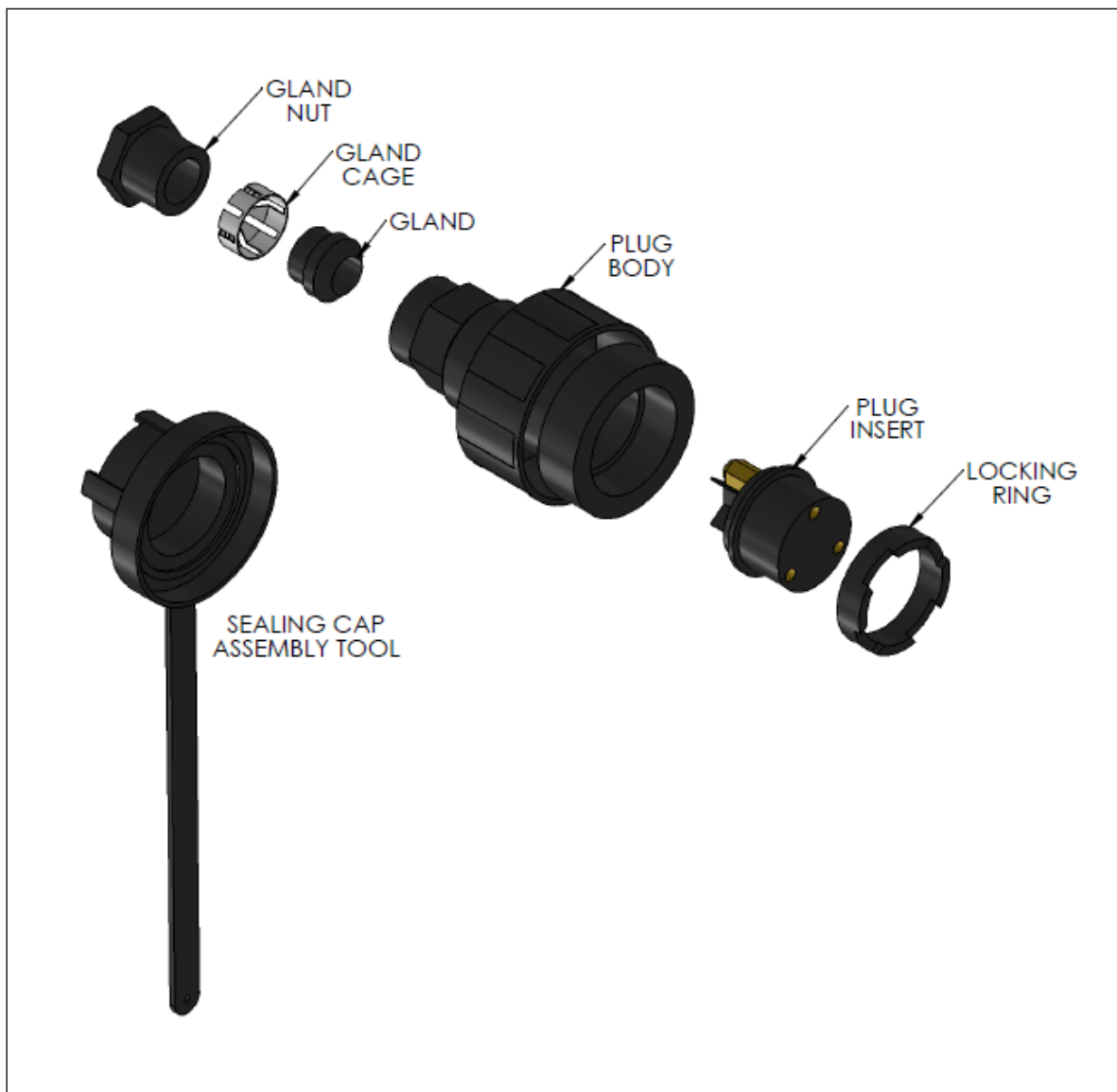
Figure 15. Disassembled Plug Connector
