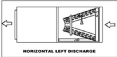
Fig 6A-1 - Air flow direction in Horizontal Left application
